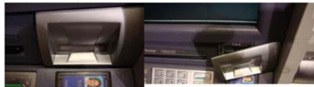
Skimmer placed over card slot & Partially removed
