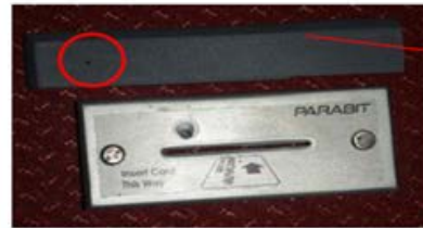
Door Access Device Skimmer & PIN Capturing Device
