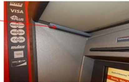
Location of PIN capturing Device camera (Usually placed somewhere above PIN pad)
