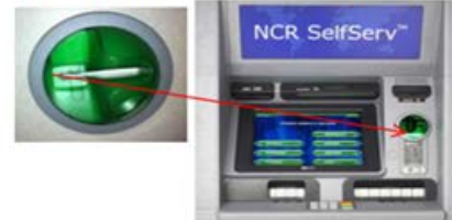
Skimmer placed over the original card slot of the ATM
