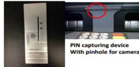
Counterfeit Door Access Device Placed over original door access Device by lobby door entrance
